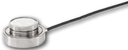
47AX is a low profile 1/2" precision pressure microphone set with built-in CCP preamplifier. With a height (to the diaphragm) of only 8 mm, 47AX is suitably designed for flush mounting in plates in ground array applications and other applications with size constraints.
