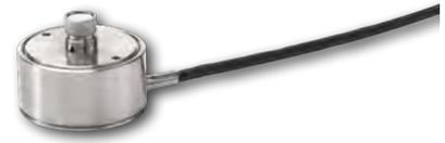
47DX is a low profile 1/8" precision pressure microphone set with built-in CCP preamplifier. With a height (to the diaphragm) of only 9 mm, 47DX is suitably designed for flush mounting in plates in ground array applications and other applications with size constraints.
