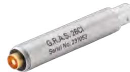
26CI is optimized for low frequency use with prepolarized condenser microphones. It uses a CCP power supply (ICP ©), e.g. 12AL. It has a very low inherent noise level, a large dynamic range and a frequency response from 1 Hz to above 200 kHz.
