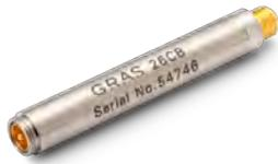
26CB is a CCP preamplifier with integrated Microdot connector for use with 1/4" prepolarized microphones. It includes built-in TEDS which enables it to be programmed as a complete unit together with a microphone.
