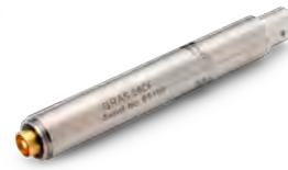
26CF is a CCP preamplifier with integrated BNC connector for use with 1/2" prepolarized microphones and standard constant-current input devices. It has two flush-mounted switches for selecting various combinations of gain and filtering, i.e.:
