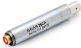
26CA is a CCP preamplifier with integrated BNC connector. For use with 1/2" prepolarized microphones and standard constant-current input devices. Includes built-in TEDS which enables it to be programmed as a complete unit together with a microphone.
