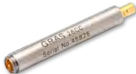
26CC is a CCP preamplifier with integrated SMB connector. For use with 1/4" prepolarized microphones. For direct use on GRAS Array Modules PR0001 and PR0002 connected to constant-current input devices. Includes built-in TEDS which enables it to be programmed as a complete unit together with a microphone.
