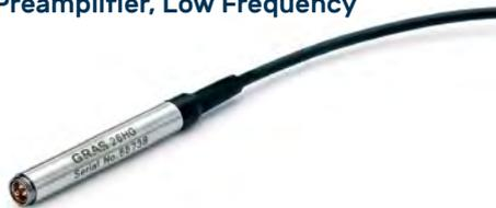
Similar to 26AC but with 40 GΩ input impedance to enable low level and low frequency measurements. It has a 3 m integrated cable.
