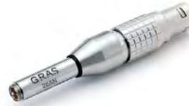
Preamplifier with an integrated 7-pin LEMO connector. Configured to permit use of the insert voltage technique for determining the open-circuit sensitivity of a microphone. A 1/4" to 1/2" adapter, GR0010, is included, so that it can also be used with GRAS 1/2" microphones. Cable is not included.
