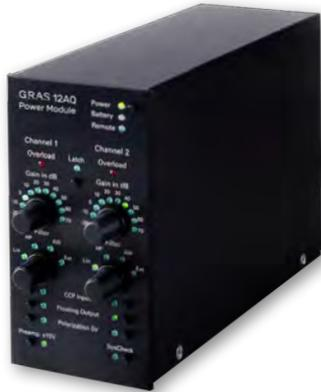
12AQ is a 2-channel power module for powering microphone preamplifiers requiring a constant-current or constant voltage power supply. 12AQ is for general use in acoustic measurements as well as for intensity measurements, both in the laboratory and in the field. It has facilities for both manual control and remote control. Manual control is via front-panel switches and push buttons. Remote control is via RS-232 interface.
