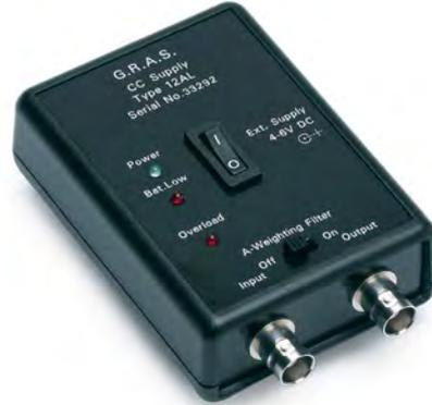
12AL is a 1-channel CCP Power Module for powering microphone preamplifiers requiring a constant-current power supply, e.g. 26CB and 26CA. It can also power the 40SC Probe Microphone as well as the 40PH and 40PL Array Microphones.
