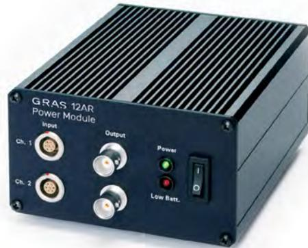
12AR is a 2-channel, battery-operated, microphone power module. It has two 7-pin LEMO 1B input connectors for microphone preamplifiers and two BNC output sockets. It can provide a polarization of 200 V for externally polarized or 0 V for prepolarized microphone cartridges.
