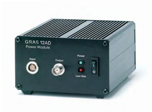
12AD is a 1-channel, battery-operated, microphone power module. It has a 7-pin LEMO 1B input connector for a microphone preamplifier and one BNC output socket. It can provide a polarization of 200 V for externally polarized or 0 V for prepolarized microphone cartridges.
