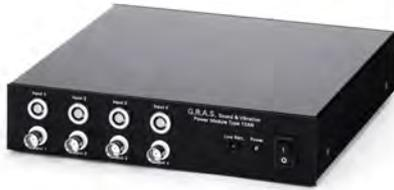
12AN is a 4-channel power module for general use. It is a cost-effective solution with direct coupling (no filters), and is therefore ideally suited for infra-sound measurements. It can be used with all standard LEMO microphone sets and standard front-ends or acquisition units.
