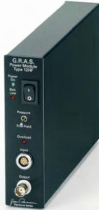
12HF is a power module for single-channel, low-noise measurements using the matched, low-noise preamplifiers and high sensitive microphones of 40HF, 40HH and 40HT Low-noise Microphone Systems.
