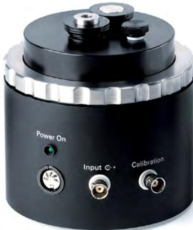
42AE permits microphone calibration at frequencies down to 0.01 Hz for both front- and rear-vented microphones.
