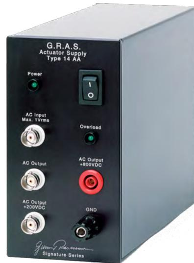
High voltage, high gain amplifier and voltage supply for driving electrostatic actuators. The high voltage output can also be used to drive standard microphones as sound sources. The 14AA can drive an electrostatic actuator with a 300 V peak-to-peak signal superimposed on 800 V DC.
